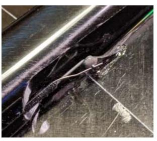
11) Put horns and springs in H and V stabs. Use a piece of masking tape over the hinge gap to keep them flat (or install springs later).
